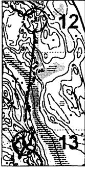
The receiver was set to log fixes i.e. locations every second while Jan was taking himself around the 7.0 km course with 16 controls. The PDOP mask (Positional Dilution of Precision) was set to 8 (accuracy degrades as PDOP increases).
